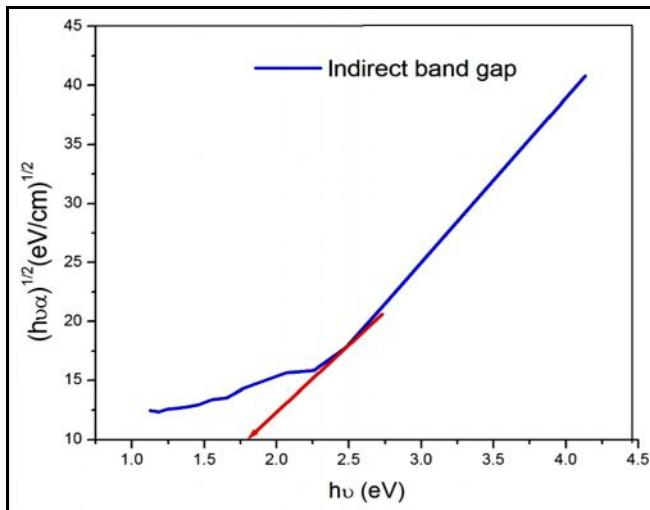
**Figure 6.** Tauc's plot of CuO nanoparticles (indirect band gap)
