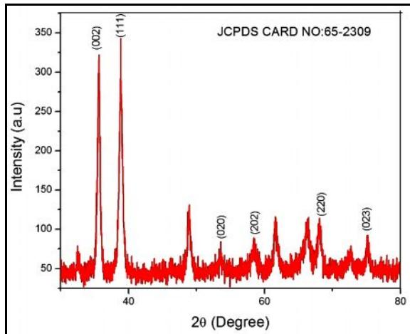
**Figure 1 . XRD Pattern of CuO Nanoparticles**
