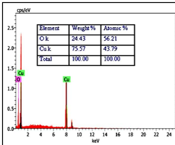
**Figure 2. EDAX Spectrum of CuO nanoparticles**
