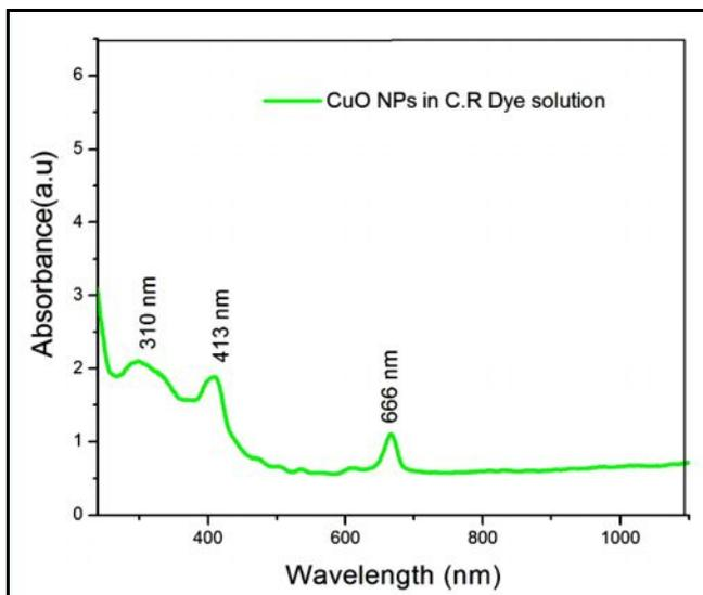
Figure 4. UV-Visible Spectrum of CuO
