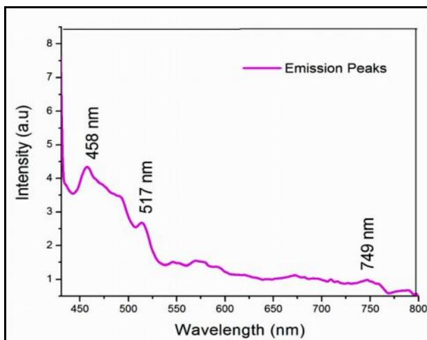
**Figure 7.** Luminescence Spectra for CuO nanoparticles in C.Roseus Dye solution
