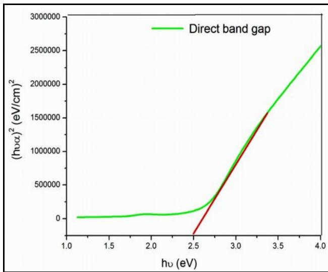
**Figure 5.** Tauc's plot of CuO nanoparticles (direct band gap)
