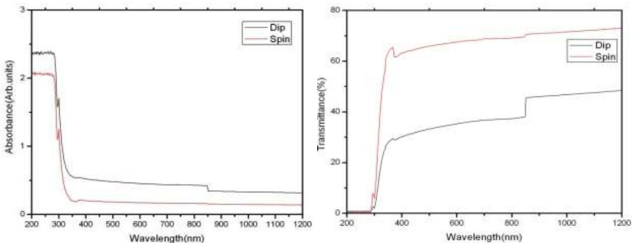
**Fig 3 The Absorbance & Transmittance spectra of a as deposited ZnS thin film**
