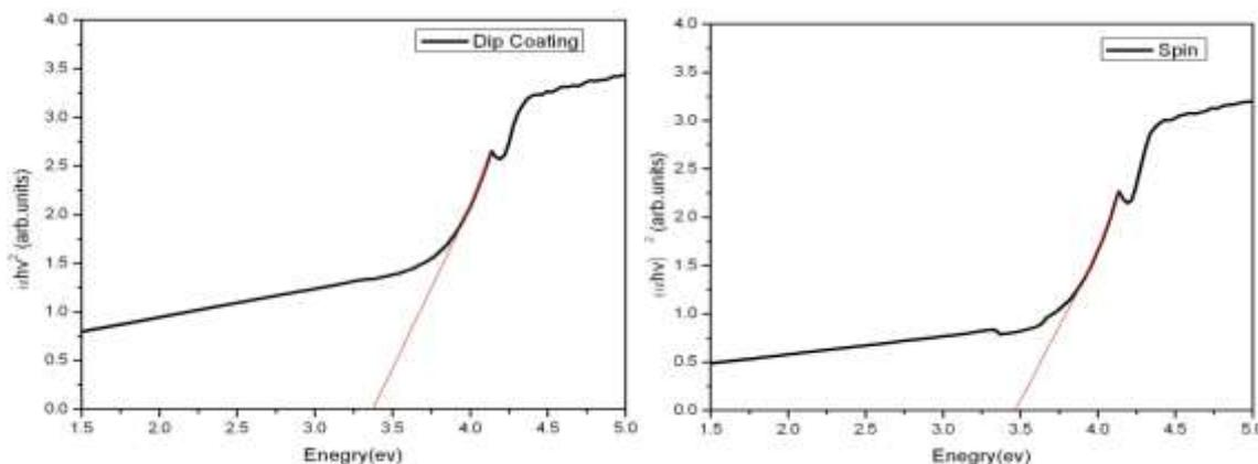
**Fig. 4.** Plot of  $(n)^2$  with respect to photon energy.
