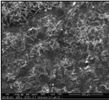
**Fig 2 SEM Micrograph of as prepared ZnS thin film**
