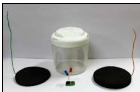
Figure 1: The anode (with green wire), cathode (orange wire), the vessel and the electronic setup.
