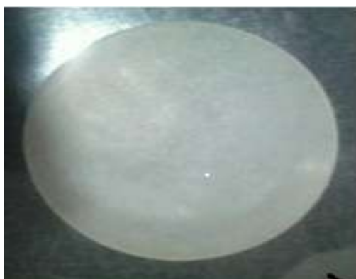
Fig 1: PAN Complexed Gel polymer Electrolyte film with NaF salt
