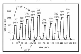
Fig.9. Repeatability of the sensor with response and recovery cycle
