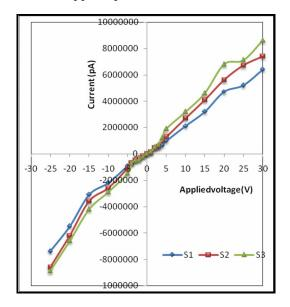
Fig. 4. I-V characteristics of nanostructured CdO thin film.
