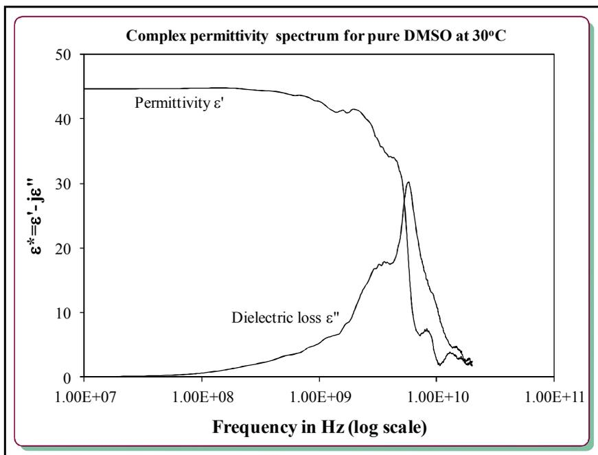
Figure 1: Typical plot showing variation in permittivity with frequency for pure DMSO at  $30^\circ\text{C}$
